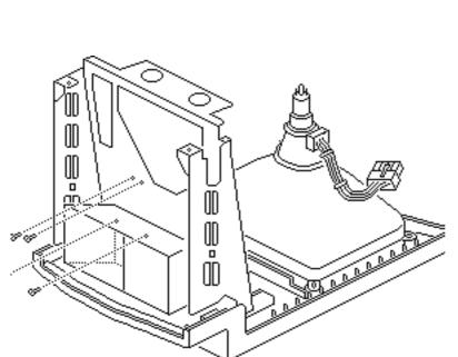
1 Remove the four Phillips screws that secure the floppy drive housing to the bottom of the chassis.
