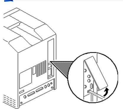
2 Using a small flat-blade screwdriver, depress the center tab and lift out the service door.
