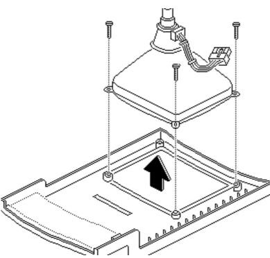
Remove the three Torx screws from the corner of the CRT, and remove the CRT.
