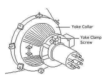
Note: If glue holds the yoke collar in place, use an art knife to cut through the glue.
