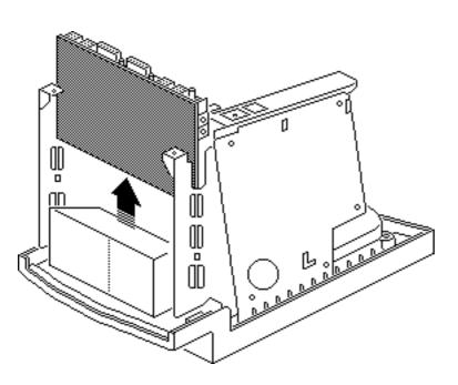
Grasp the logic board by the corners and slide it straight up and out of the chassis.
