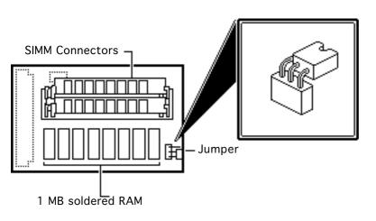
Note: Install the memory board without additional SIMMs for a 1 MB RAM upgrade. Install two 256K SIMMs onto the memory expansion board for a 2.5 MB RAM upgrade or two 1 MB SIMMs for a 4 MB RAM upgrade.
