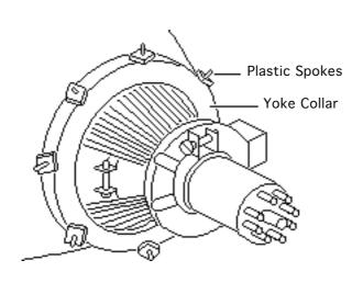
3 With one hand, grasp the plastic spokes of the yoke collar and rotate the yoke collar until the top and bottom edges of the picture are parallel with the top and bottom of the bezel.
