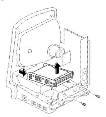
Remove the two Phillips screws that secure the hard drive housing to the floppy drive housing and lift out the hard drive assembly.
