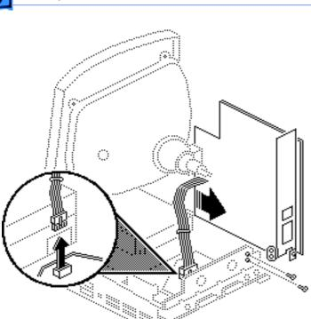
3 Remove the logic board power cable from the logic board. Remove the Phillips screws that secure the power/sweep bracket to the chassis and pull the board slightly away from the chassis.
