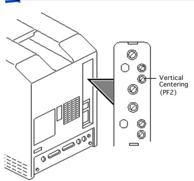
4 Using the plastic hex alignment tool, adjust the vertical centering control to center the image vertically within the bezel.
