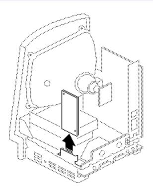
**Note:** The memory expansion board is an option for the Macintosh Classic only. It contains 1 MB of soldered RAM plus one pair of SIMM connectors.
