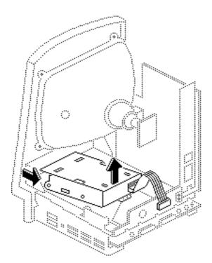
2 Lift out the floppy drive mechanism.
