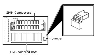
**Note:** The memory expansion board is an option for the Macintosh Classic only. It contains 1 MB of soldered RAM plus one pair of SIMM connectors. You can upgrade the system further by adding two 256K or two 1 MB SIMMs to the memory expansion board and moving the jumper. You must use 120-ns (or faster) SIMMs.
