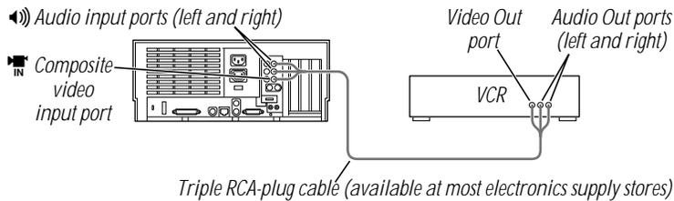
**S-video connection for input from a camera**
