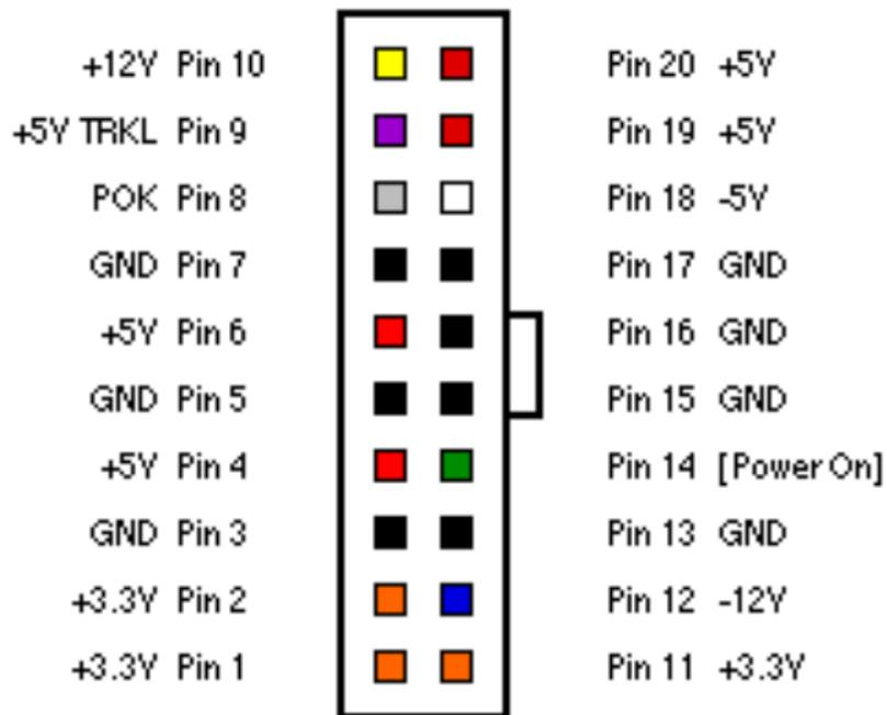
Figure 1. Power Supply 20-Pin Connector
