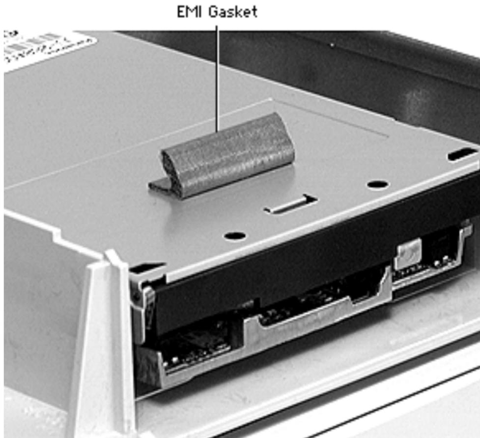
**Replacement Note:** When replacing the floppy drive, you must install an EMI gasket (p/n 922-1895). Peel off the adhesive and attach the gasket in the center of the drive's top surface, with the "V" of the gasket pointing at the front edge of the drive.
