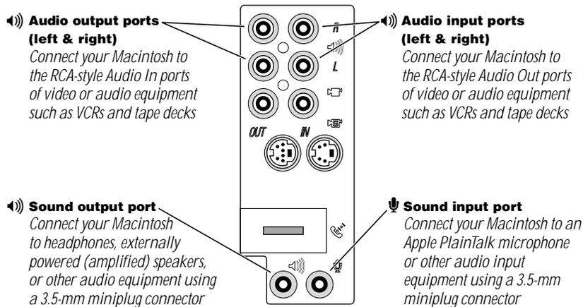
The left and right RCA-type ports accept this type of connector:
