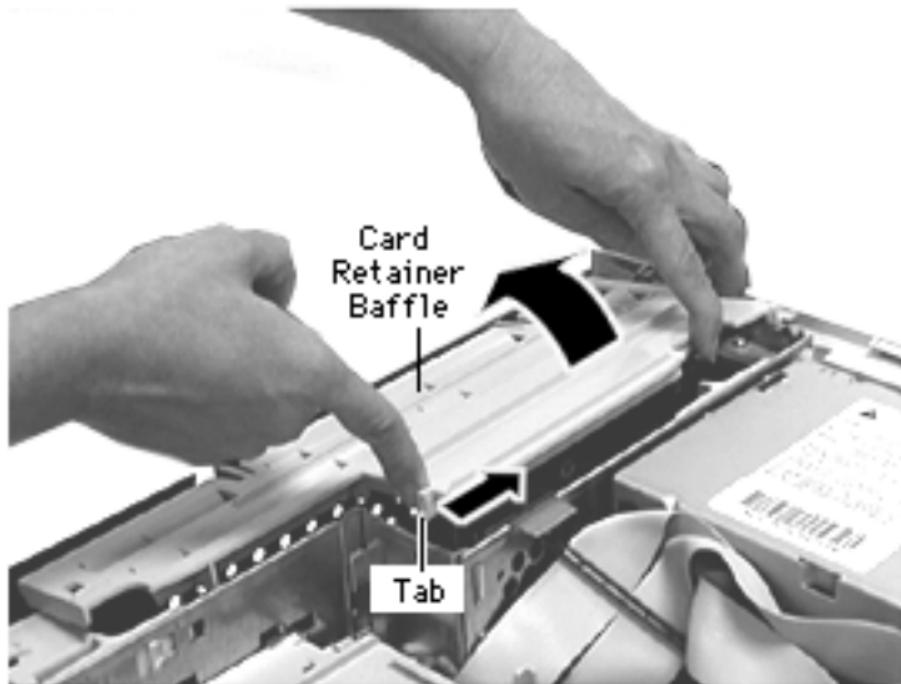
**To Open the Card Retainer Baffle:**
