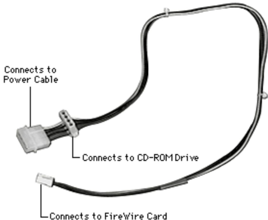
**Note:** The graphic at left shows the internal FireWire cable and each of its connectors.
