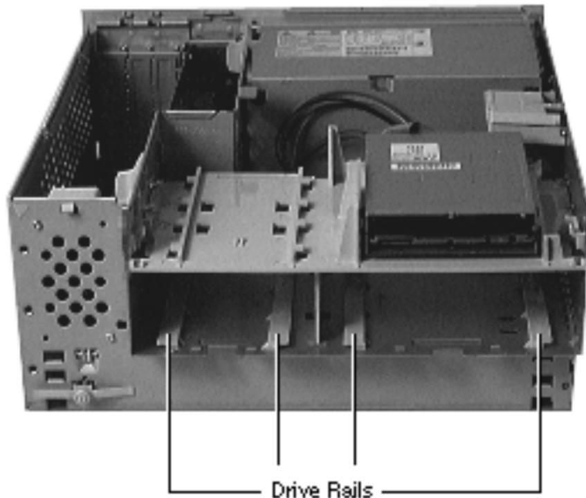
**Note:** The drive rails attach to the chassis underneath the CD-ROM or DVD-ROM drive, Zip drive, and hard drive.
